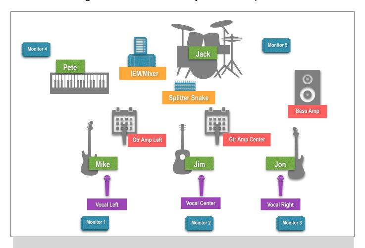
Band Controlled In-Ear Monitor Mixer Inputs with Fan-tail/Splitter Snake (Band Provides) Drums are Triggered Electronic Kit with Left and Right XLR Outputs on Mackie 1000w (Roland TD 15 connected to 2 Mackie 1000W Powered Speakers)
